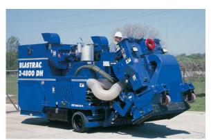
The front end lift system raises the blast head for transport
